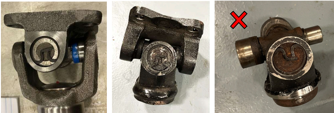
Above: 1. A new U-joint. 2. Good U-joint – clean and sealed with smooth rotation. 3. Bad U-joint – Rusted out with gritty motion and/or slop in the joints.
