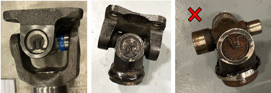
Above: 1. A new U-joint. 2. Good U-joint – clean and sealed with smooth rotation. 3. Bad U-joint – Rusted out with gritty motion and/or slop in the joints.
